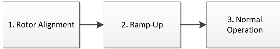
Figure 2 - Sensorless drive startup steps
