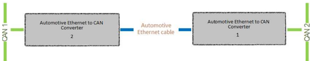
Figure 22. Simple Local Connection
